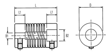
B1: Pre-drilled = 3.0B2: Pre-drilled = 5.00D = 12.7L = 25.4L1 = 6.5Max angular displacement = 0.17Max B1 & B2 = 6.35Max parallel displacement = 5 Peak Torque NM = 3.00 Set Screw = M3
